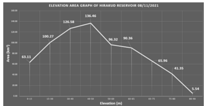
Fig.10 (a, b, c, d, e): Elevation-Area curve of Hirakud reservoir (1990, 2000, 2010, 2020, 2021)
