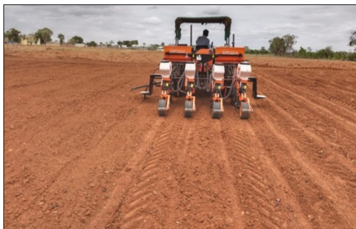
Fig 5. Precise sowing of cotton with vacuum planter
