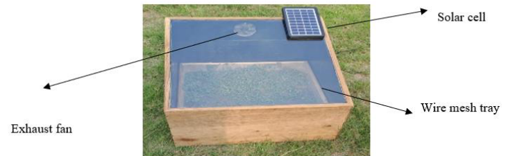
Fig 3: Experimental set up direct Solar dryer
