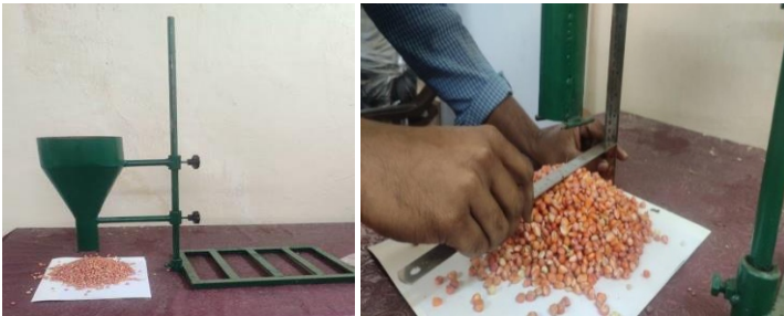
Fig.2. Measurement of angle of repose
