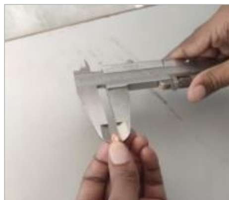
Fig 1. Measurement of size by using Vernier caliper
