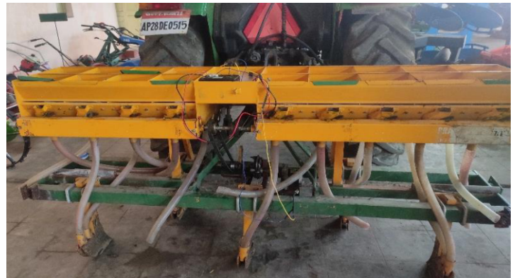
Fig.8. Microcontroller unit attachment to planter
