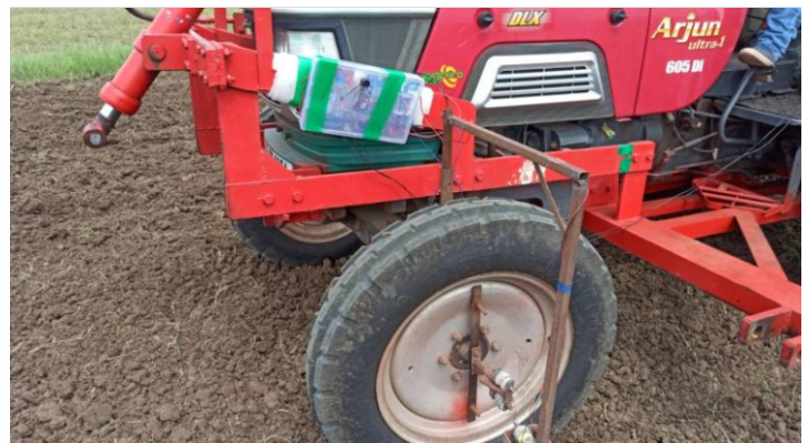
Fig.7. Wheel RPM sensor attachment to tractor front wheel
