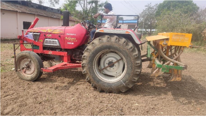
Fig.9. Developed Microcontroller Operated Planter
