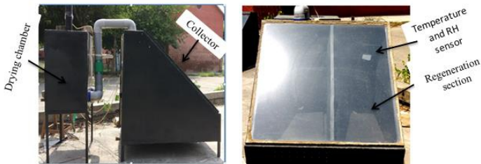
Fig 1: Experimental setup of the developed desiccant-assisted automated hybrid solar dryer
