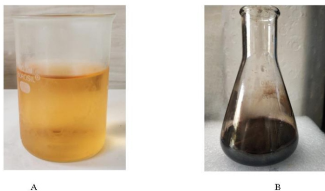
Figure 1: Colour change indicating formation of silver nanoparticles (A) Extract (B) Prepared nanoparticles
