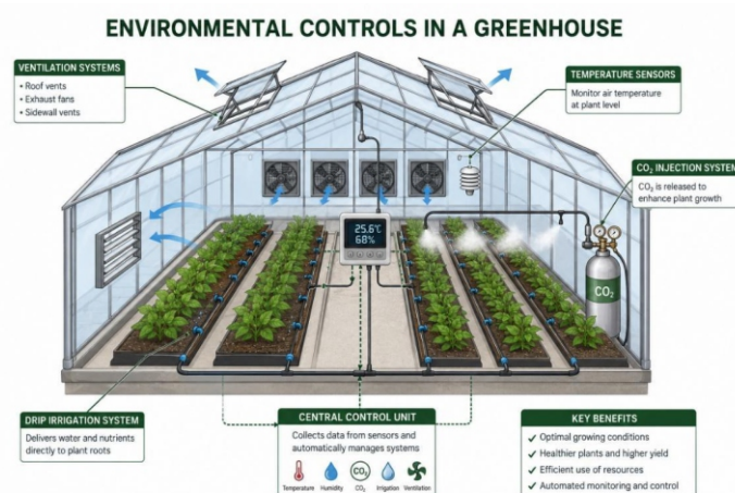
Figure 4: Schematic representation of automated environmental control systems within a modern greenhouse
