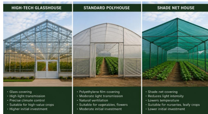
Figure 3: Structural and functional comparison of high-tech glasshouses, standard polyhouses and shade net houses
